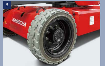
3 Tires: foam-filled tires with good off-road performance
