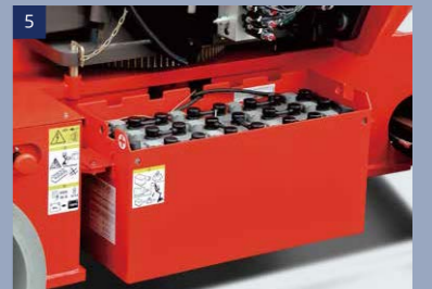
5 Standard tracking battery: Reduce 40% of the charge time, raise 50% of the life time
