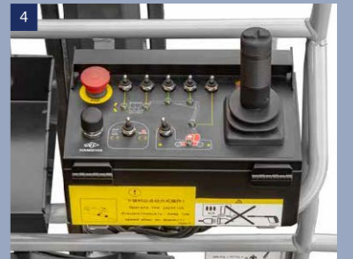
4 Basket control box: each action of the device can be controlled through the control box to quickly reach the working area, and the control is simple and easy to understand
